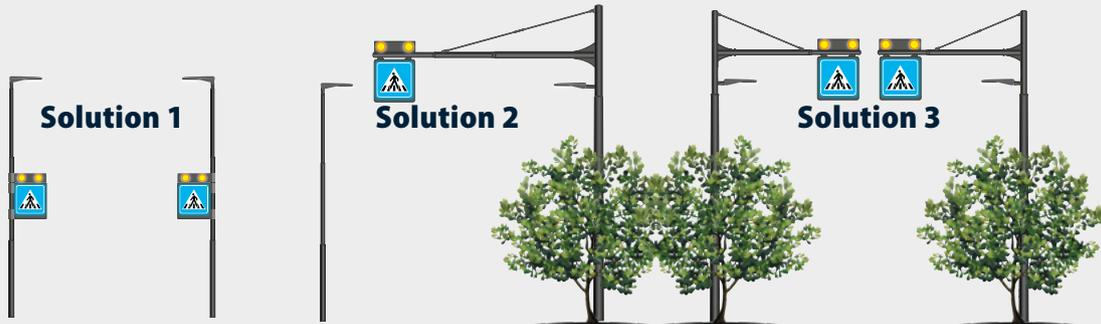
Solutions 2 and 3 are suitable for installations on roads with limits above 50 km/h (e.g. **70**)
